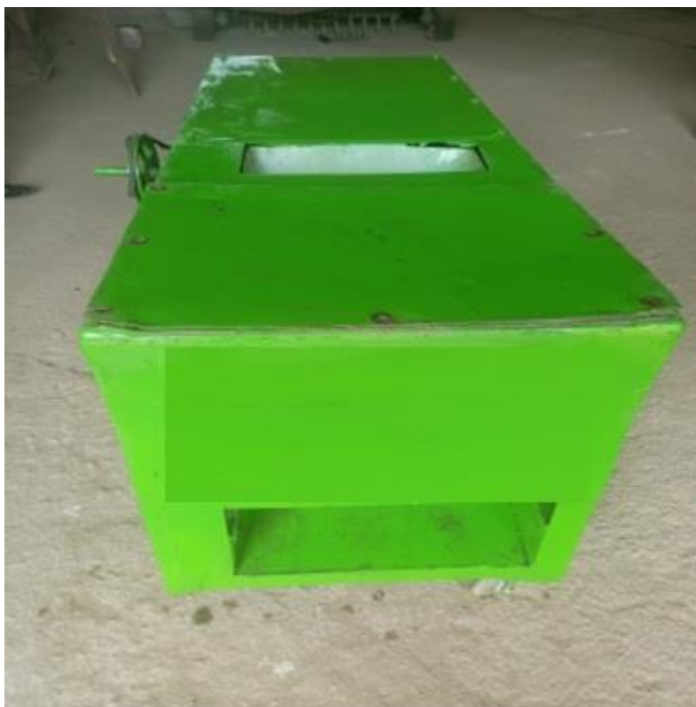
Plate 3: The yam minisett processing machine
