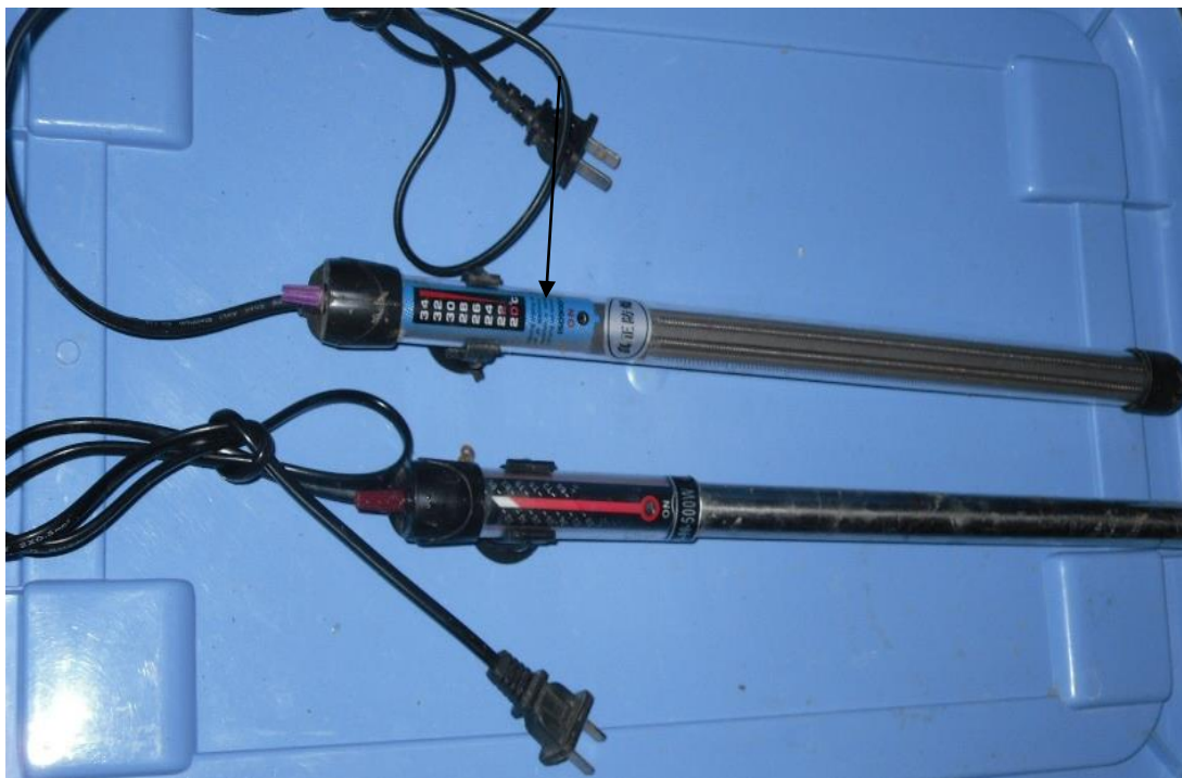
Plate 11 Thermo-regulated Heaters used in Manipulating Temperature during Growth of C. gariepinus Fingerling.
