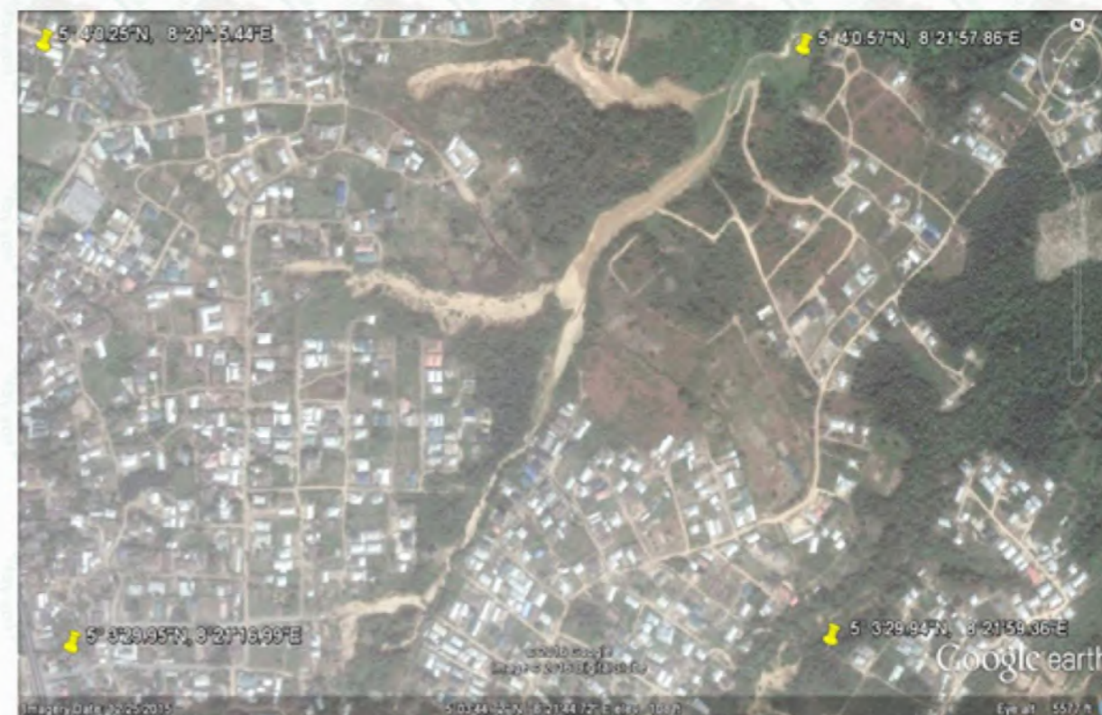
Plate 1: Satellite Imagery of the Gully Erosion Sites in Ikot Nkebre NEWMAP Project Area. Run off from gully fingers discharge into the Ikot Nkebre stream (Calabar Municipality).
